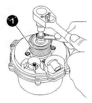
ASSEMBLING ALTERNATOR Assembling pulley Pulley cap is always to be renewed. Cap is either inserted or clipped on.
